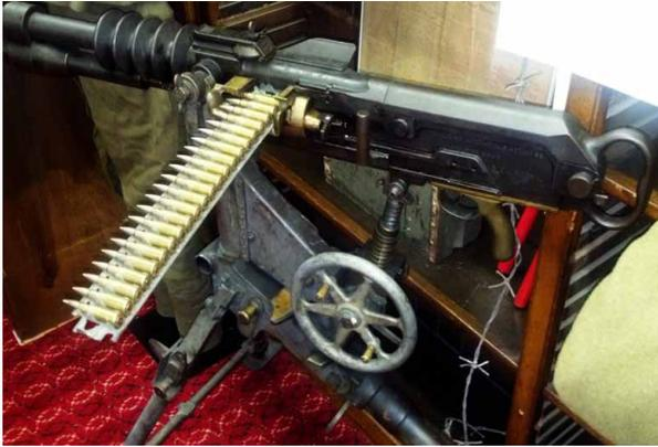
Shown here is the feed strip in place, as well as the wheel used to elevate and depress the muzzle. The tripod is made to collapse in several positions, so that the gun can be made to “kneel” and fire downward; it also has a provision for an axle and wheels to be added for pulling it. The weapon was made with simplicity in mind; it has 30 parts which can be disassembled without tools, and each part is made so that it can't be reassembled incorrectly.
